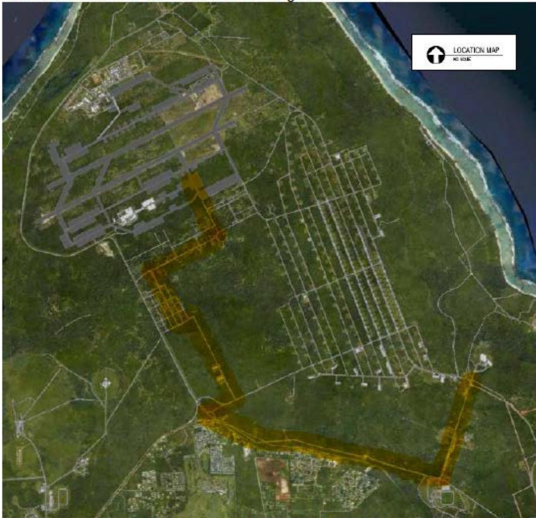
**Project will install communication lines between J-200 and the LFTRC. Approximate path is highlighted; actual APE follows existing road and utility corridors within the shaded area.**
